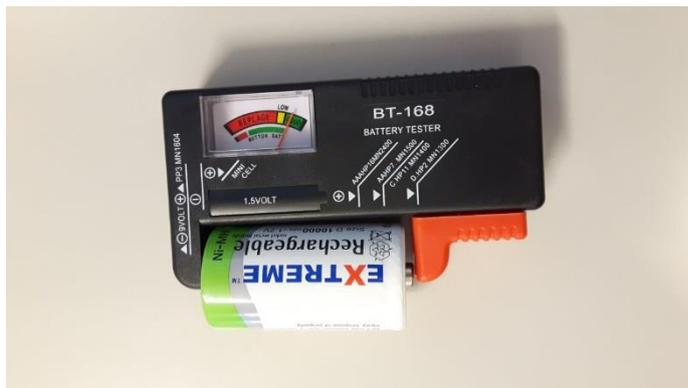
**How to test the batteries:** simply push the red slider as far to the right as it will go, and insert the battery into the space (with positive charge on the right, next to the slider). Read the display to check that it says 'good'.
